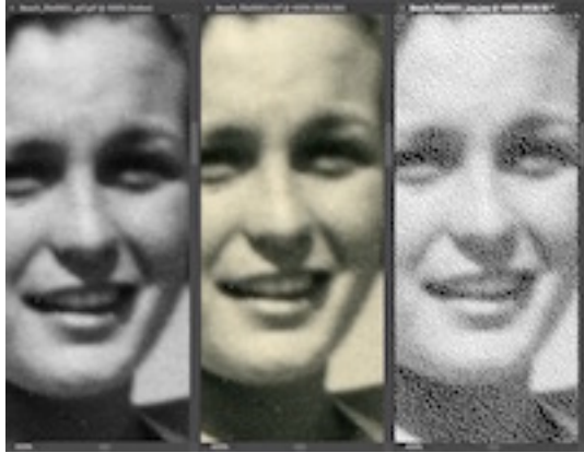
Figure 1. Compression artifacts are apparent in the JPEG version (right) when viewed at 400%.
