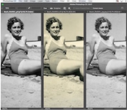
Figure 3. The GIF (left) and the TIFF (middle) files look similar when viewed at 66.67%. However, the JPEG (right) file begins to look pixilated.
